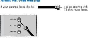
Plug the antenna lead into the "ANT 1 IN" terminal on the rear panel.
